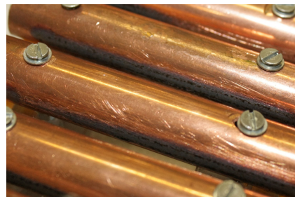
Figure 4.24: Heavy corrosion between the copper tubes.
