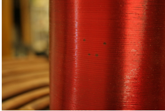
Figure 4.29: Results of inadequate space between the coils : arcing between the two occurred, burning the secondary coil at several points.
